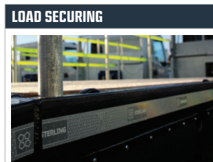
Lashing rings every 900mm Lashing rings under side rave (only on the 32T model)
