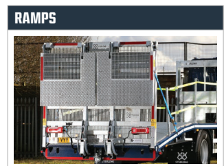
Full-width 2.5m double flip ramps
