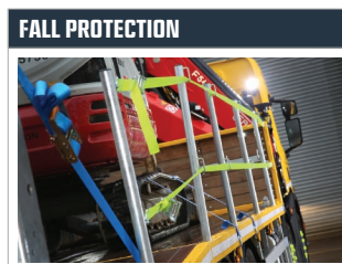
Post & Socket fall arrest with Storage tray Access steps to front nearside
