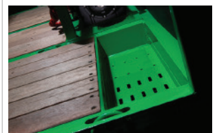
1x 1000mm plastic toolbox Recessed chain trays at front of body
