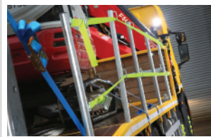
Post & Socket fall arrest with Storage tray Access steps to front nearside
