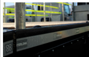
Lashing rings every 900mm Lashing rings under side rave (only on the 32T model)
