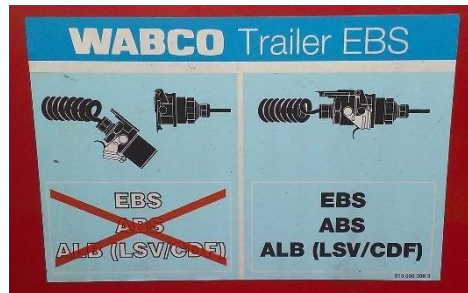
Figure 6: WABCO Trailer Brake Label
