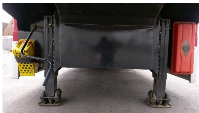
Figure 17: Example Image of Landing Legs in Lowered Position
